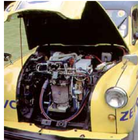
Above: In London smoking taxis have been retrofitted with fuel cell technology. South Australia is well placed for producing hydrogen for fuel cell powered vehicles. Source: Herbert Girardet
